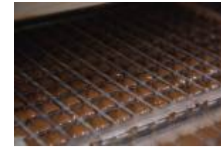
Pouring into molds to form cube shapes
